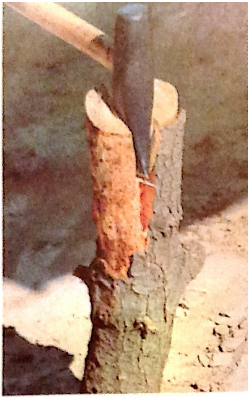
Figure 12 A large force is required to split a log in two. But with the use of a wedge, a small force is multiplied to do the job.
